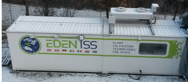
Figure 11: Mobile Test Facility with roof-mounted free cooler.
