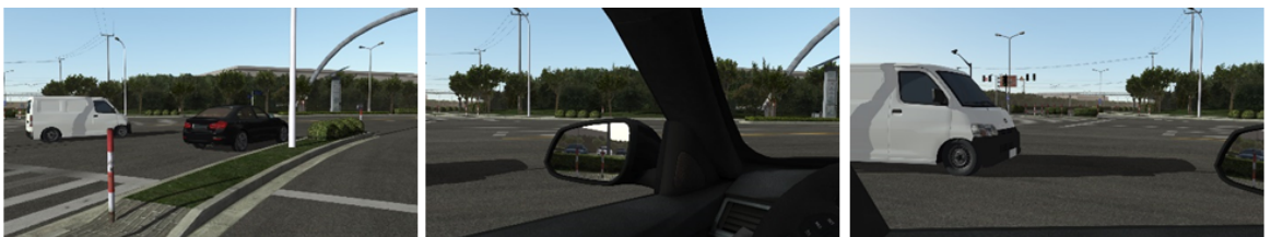
Figure 4.10: SUMO controlled traffic in the "blind spot" of a human controlled ego vehicle at a filter lane
