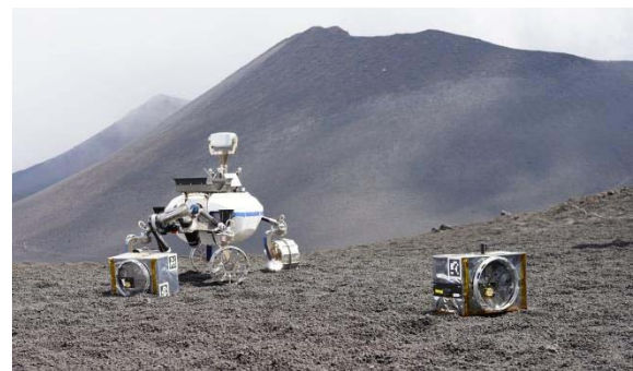
Fig. 16: The LRU rover during the deployment of the seismic instrument on Mt. Etna, Sicily.
