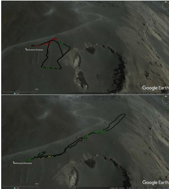
Fig. 14: Google earth view of the two tracks extracted from the DGPS data collected as ground truth (top: 796m and bottom: 1184m )
