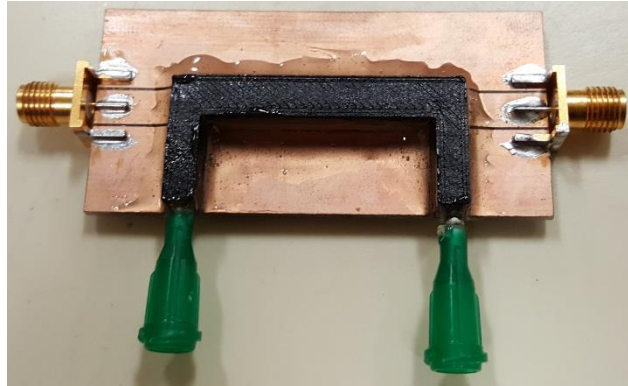
Figure 13. Fabricated H-Slot Filter with 3D-Printed Fluid Channel
