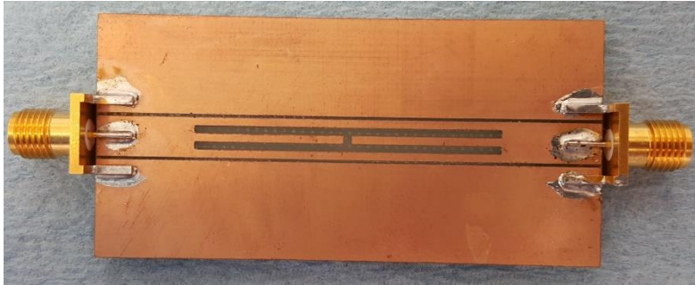
Figure 7. H-Slot Filter Fabricated on 62 mil FR-4 ( \epsilon_r = 4.4 )
