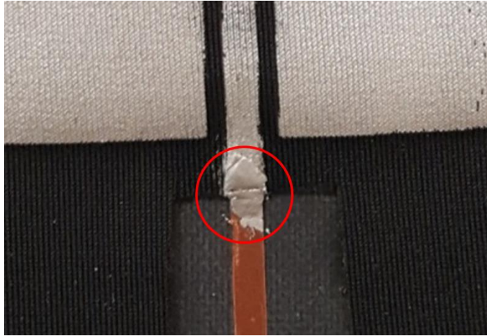
Figure 31. Feedline Junction of Fabricated Printed Metal Patch Antenna
