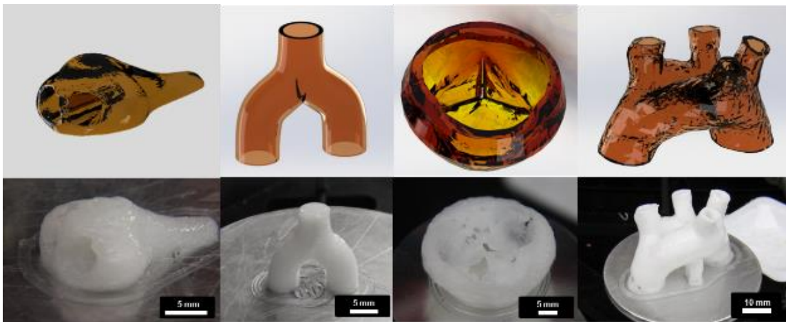
Figure 4.7. Complex anatomical models printed to demonstrate the clinical applications and versatility of these hydrocolloid inks and the extrusion CoD technology. Models printed (from left to right) include a nose, bifurcating vessel, semilunar valve, and congenital deformity of an aortic arch. Resulting printed constructs are shown below each model to demonstrate the quality and detail afforded by the hydrocolloid inks.
