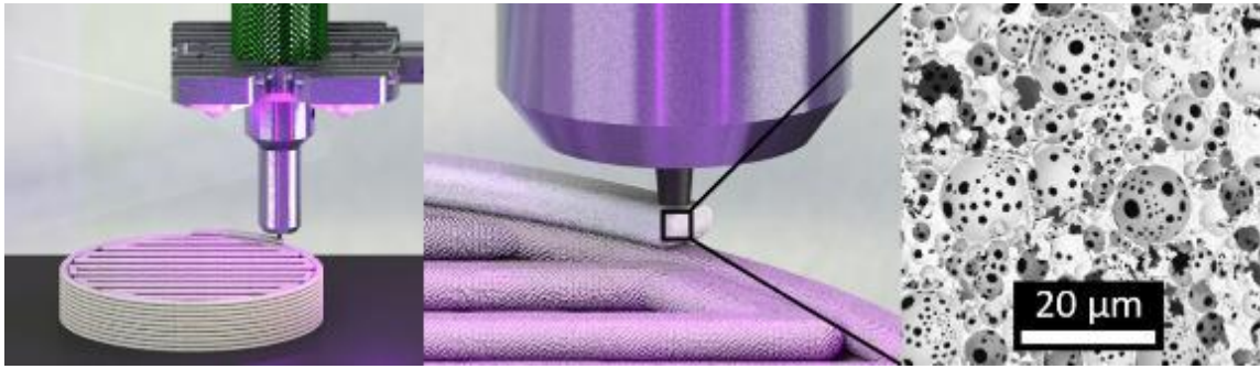
Figure 2.1. Schematic of emulsion ink printing setup with UV Cure-on-Dispense (CoD).
