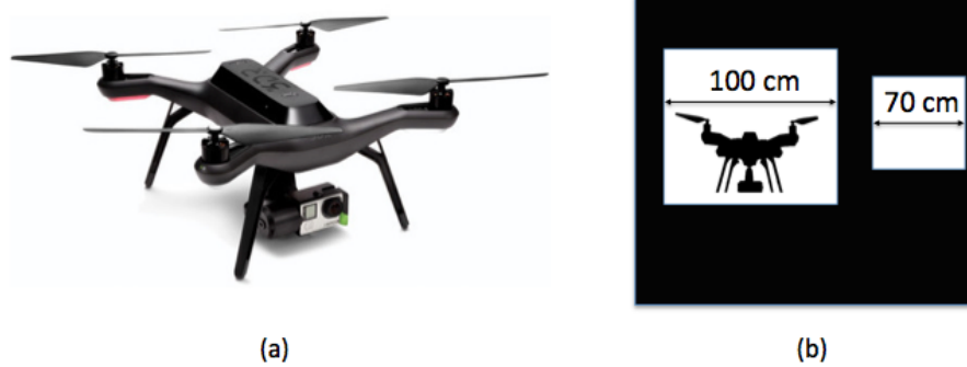
Figure 6.6: (a) 3DRobotics Solo quadrotor platform used for flight experiments (b) Illustration of fabric panel with openings cut for gaps
