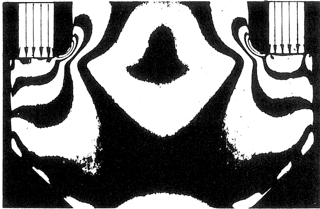
Figure 14. Stress Concentration in Fillet of T-root [3].
