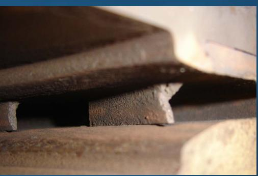
When disassembled in the workshop, the cause of the aerodynamic instability was clear: severe loss of material in both inlet and diffuser vanes of the first stage.
