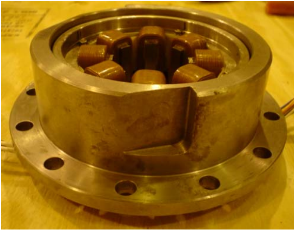
Figure 9: Magnetic Bearing Used for the Excitation
