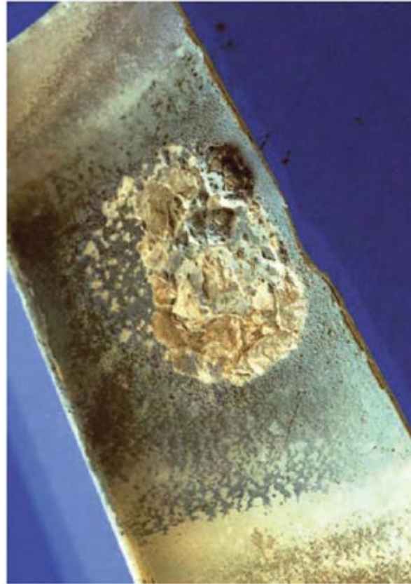
Figure 17: Accelerated Surface Oxidation Caused by Vanadium in Heavy Fuel Oil (Courtesy, Turbotect Ltd.)
