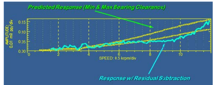
Figure 10) 8 Stage Compressor – Measured vs. Predicted Verification Response
