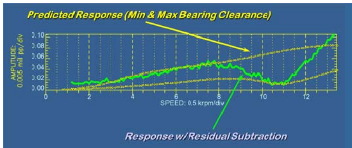
Figure 12) 3 Stage Compressor – Measured vs. Predicted Verification Response
