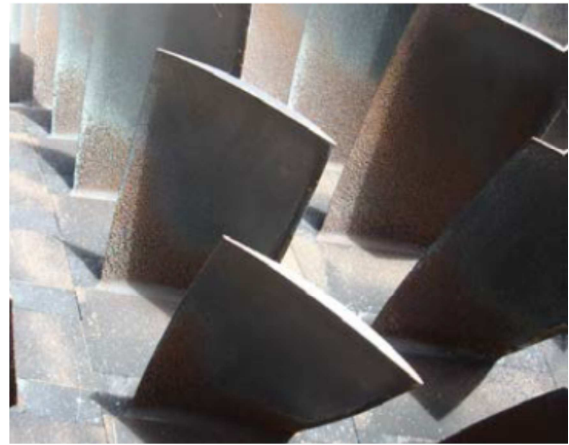
Figure 12: Axial Compressor Corrosion.
