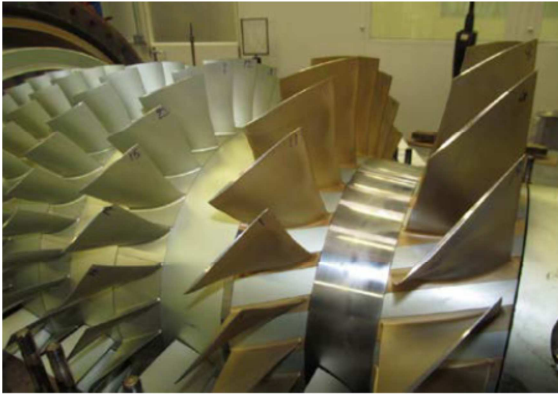
Figure 30: Same Axial Compressor after 5300 Running Hours with E12 Air Filtration.
