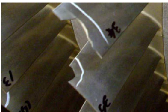
Figure 15: Tip Clip on Axial Compressor Blades.
