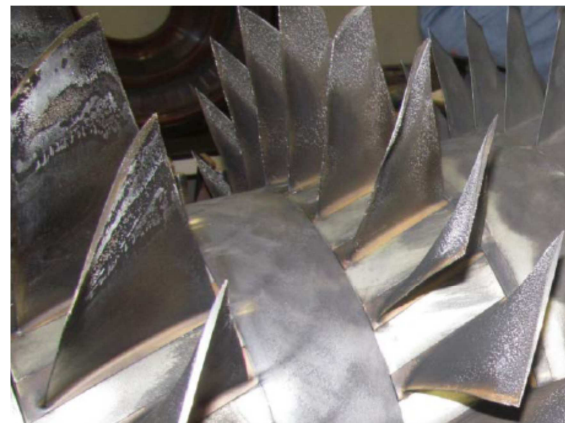
Figure 29: Axial Compressor after 4000 Running Hours with F6 Air Filtration.
