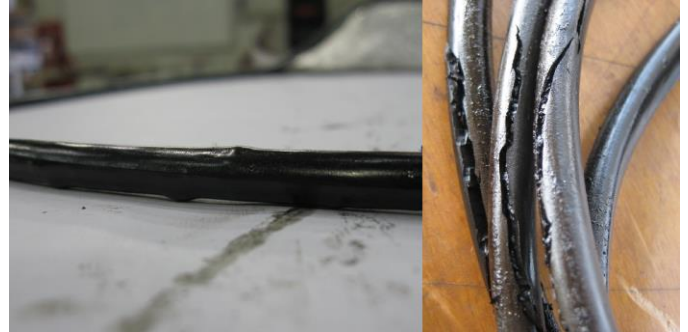
Figure 23 – The process of ED damage begins with visible bubbling of the O-ring (left) that eventually tears (right). Suggest making this two separate figures.
