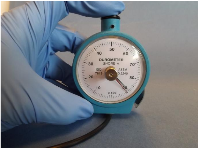
Figure 16- Portable elastomer hardness testing device.
