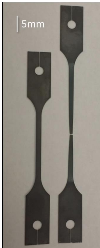
Figure 6.3: Comparison of equiatomic NiTi dogbone actuators; virgin specimen on left, fatigued specimen on right.
