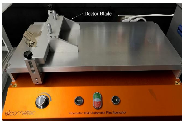
Figure 39: Automatic film applicator and doctor blade for coating slurry on a substrate.
