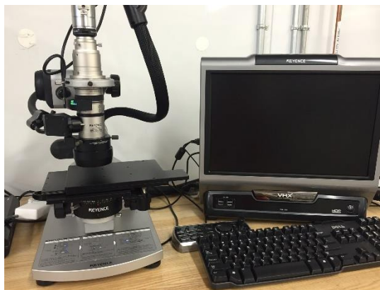
Figure 12: Optical microscope used to collect time-lapse images of the drying electrode coatings.
