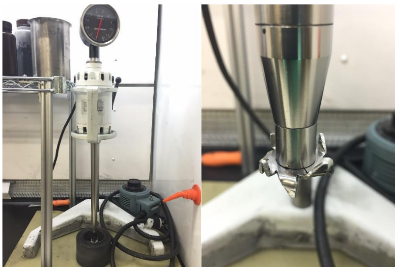
Figure 11: High shear mixer used to mix the electrode slurry ( left ), and a close up image of the mixing mechanism ( right ).
