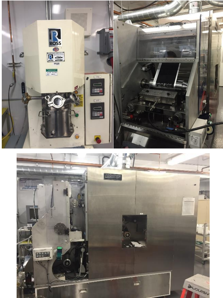
Figure 13: (Left) Planetary mixer used to mix large quantities of slurry for the slot die coater (middle). (Right) A side view of the slot die coater showing the space in which the heated drying zone is contained.
