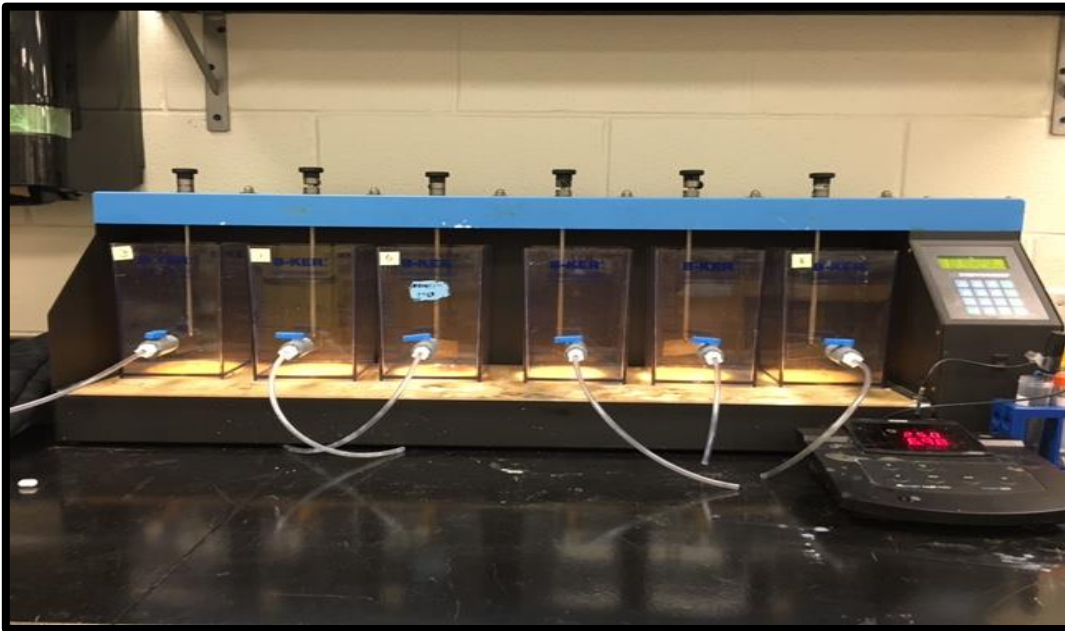
Figure 9. The programmable Phipps and Bird jar tester used for all experiments.
