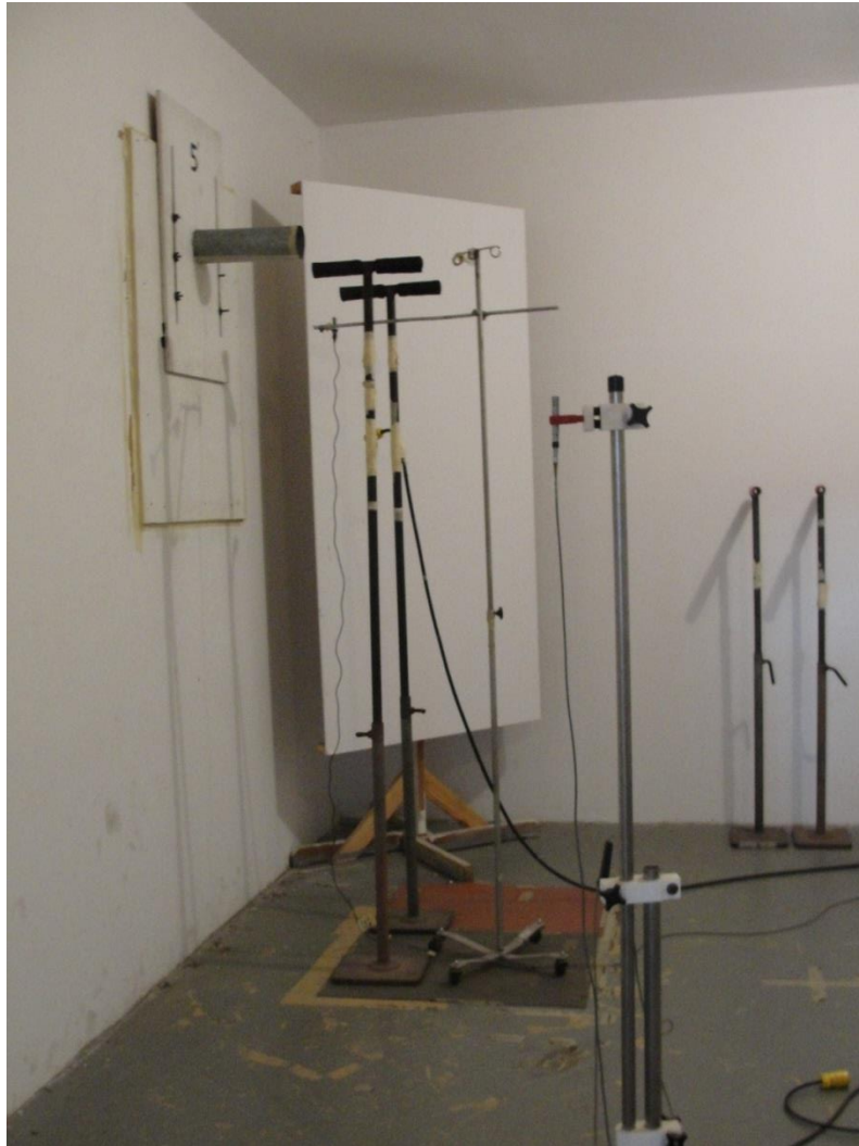
Figure 7: Sound Chamber Fan Mounting Area
