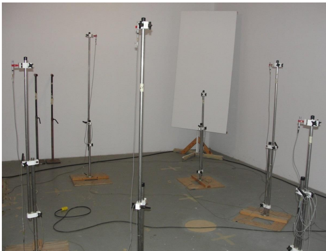
Figure 6: Sound Chamber Six Microphone Array
