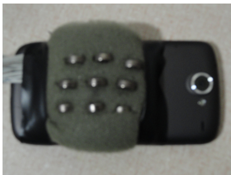
Figure 6.2: Tactor array attached to rear side of HTC Android phone.
