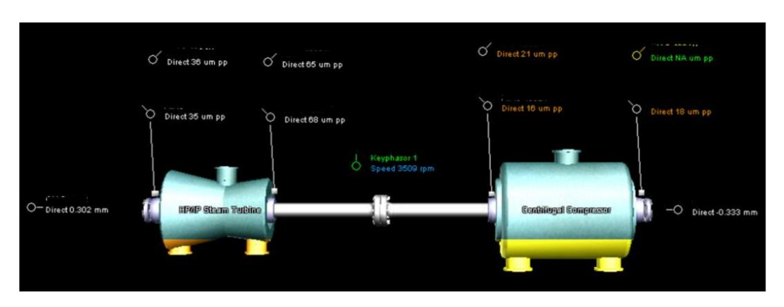
**Turbine Type** Condensing Type Impulse Reaction (11 stages)
