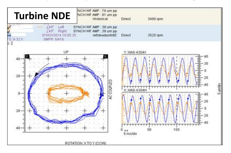
Significant change in the orbit shape and amplitude due to change in balance condition due to thermal bow.
