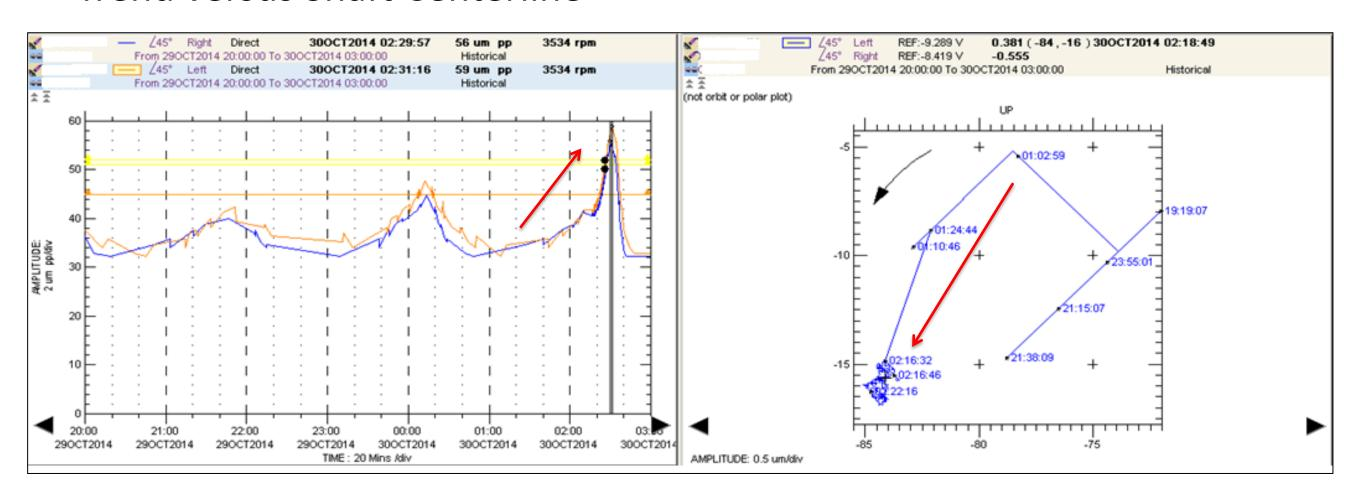
Minor change in shaft centerline noticed with the vibration increase
