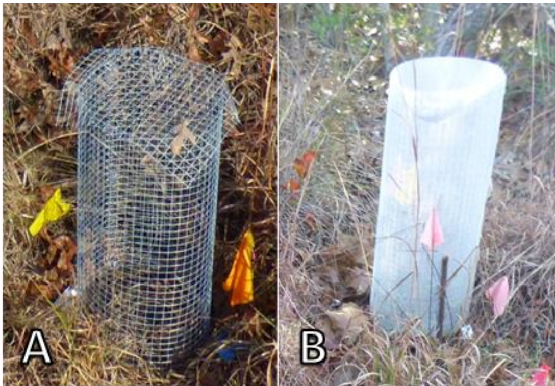
Figure 3. Cylindrical 45 cm tall and 20 cm in diameter, 1 cm 2 galvanized wire cage (A) and the same size cage lined with off white 1 mm nylon matte tulle mesh (B).
