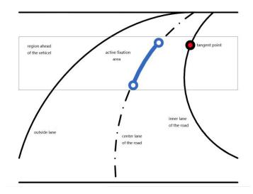
Figure 2.5: Driver Steering Fixation Area
