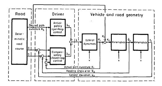
Figure 1.5: A Structural Scheme of Human Steering Behavior in the Driver-Vehicle-
