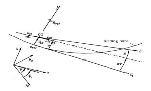
Figure 2.4: Vehicle Heading and Lateral Offset [12]
