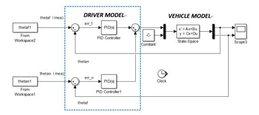
Figure 4.2: System Structure using PI Controller
