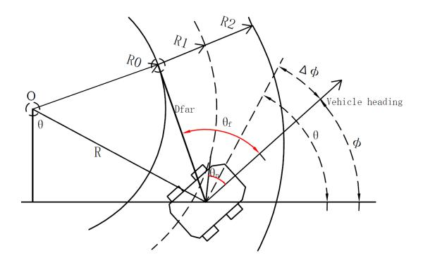
Figure 2.7: The Geometric Relationship between Vehicle and Upcoming Road
