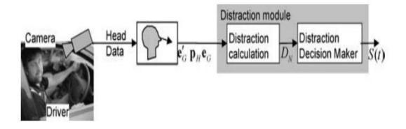
Figure 1.2: Distraction Detection Scheme [3]
