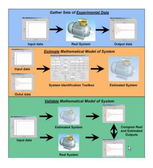
Figure 4.8 SIT Data Processing Flow [29]
