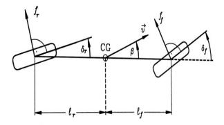
Figure 2.2: Single Track Model Equivalent Diagram [12]
