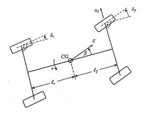
Figure 2.1: Vehicle Model with Four Wheels Steering [12]
