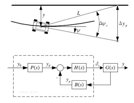
Figure 1.4: Shaft Driver Model [4]
