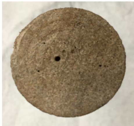
Fig. 5— Limestone core inlet after acidizing, 5 wt% HCl and 1 vol% corrosion inhibitor at 200 °F and 2 cm 3 /min.
