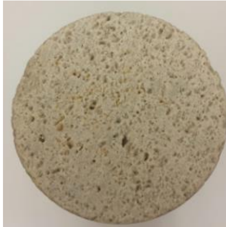
Fig. 9— Dolomite core inlet after acidizing, 5 wt% HCl and 1 vol% corrosion inhibitor at 200 °F and 2 cm 3 /min.
