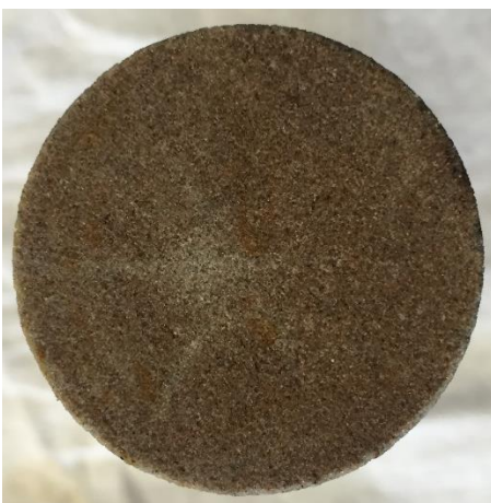
Fig. 23— Sandstone core inlet after acidizing, 5 wt% HCl, 1 vol% corrosion inhibitor and 10,000 ppm Fe(III) at 200 °F and 2 cm 3 /min (Rady and Nasr-EI-Din, 2015).
