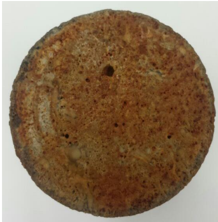
Fig. 17— Limestone core inlet after acidizing, 5 wt% HCl, 1 vol% corrosion inhibitor and 10,000 ppm Fe(III) at 200 °F and 2 cm 3 /min (Rady and Nasr-El-Din, 2015).
