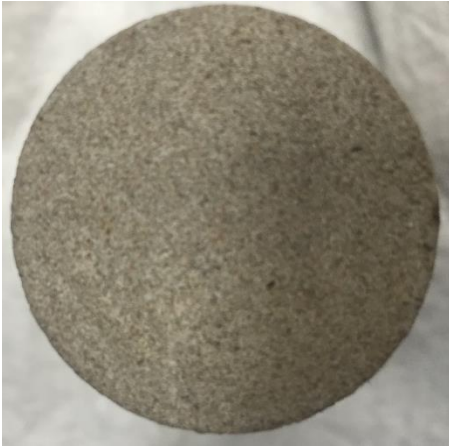
Fig. 13— Sandstone core inlet after acidizing, 5 wt% HCl and 1 vol% corrosion inhibitor at 200 °F and 2cm 3 /min.
