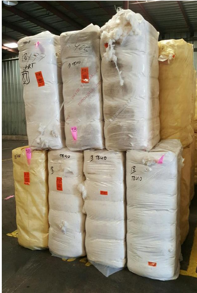
Figure 19: Bale packaging damage by hooks.
