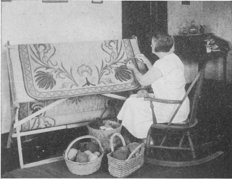
The frame into which a pattern is fastened before the process of hooking is begun is mounted on a rigid support so that the work may be done with ease and comfort. Rollers at the top and bottom of the frame allow the rug to be rolled as the hooking progresses.
