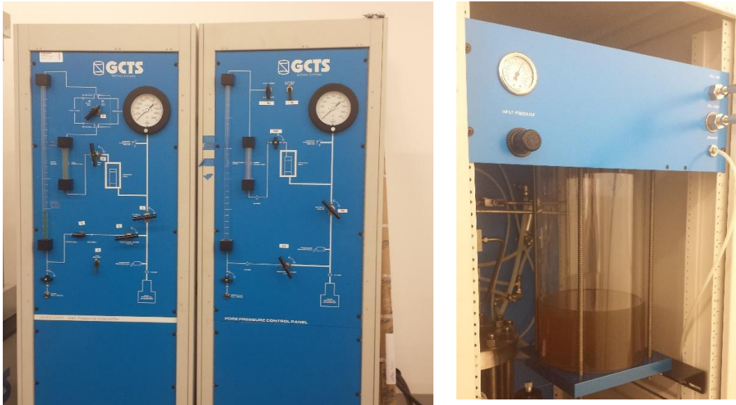
Figure 9: Cell pressure cabinet front (left) and oil reservoir (Right)
