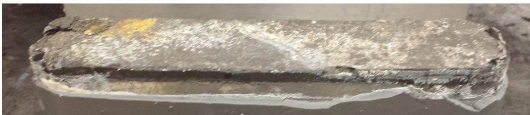
Figure 27: Fracture surface of Elmsport bed-perpendicular sample
