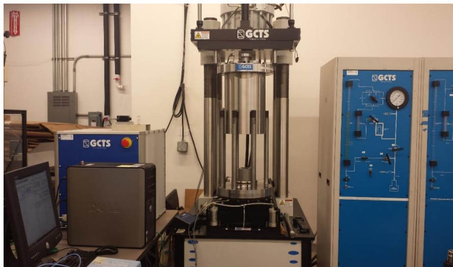
Figure 6: Experimental set up for the GCTS RTX-1500 system
