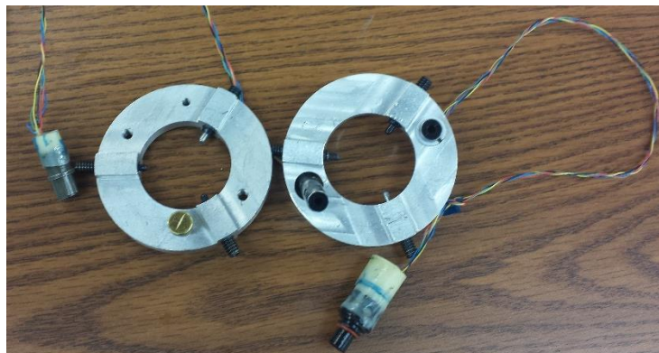
Figure 11: Metal supports for LVDT's
