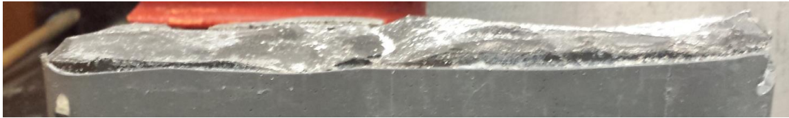
Figure 37: Fracture surface of Allenwood bed-perpendicular sample
