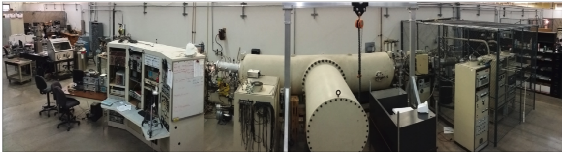
Figure 2.7: A photo of the 1.7 MV Tandem accelerator
