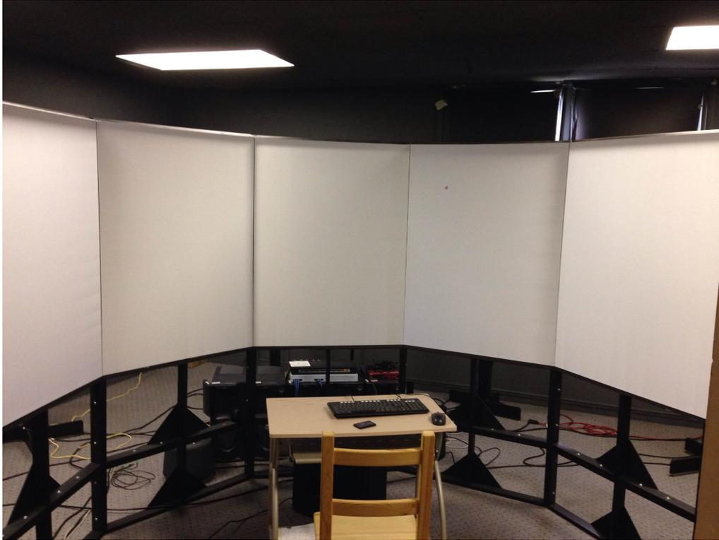
Figure 6.3: CAVE environment used in Study 1. Simulation projected on 5 screens (3600x1080) with participant interacting while seated at table.
