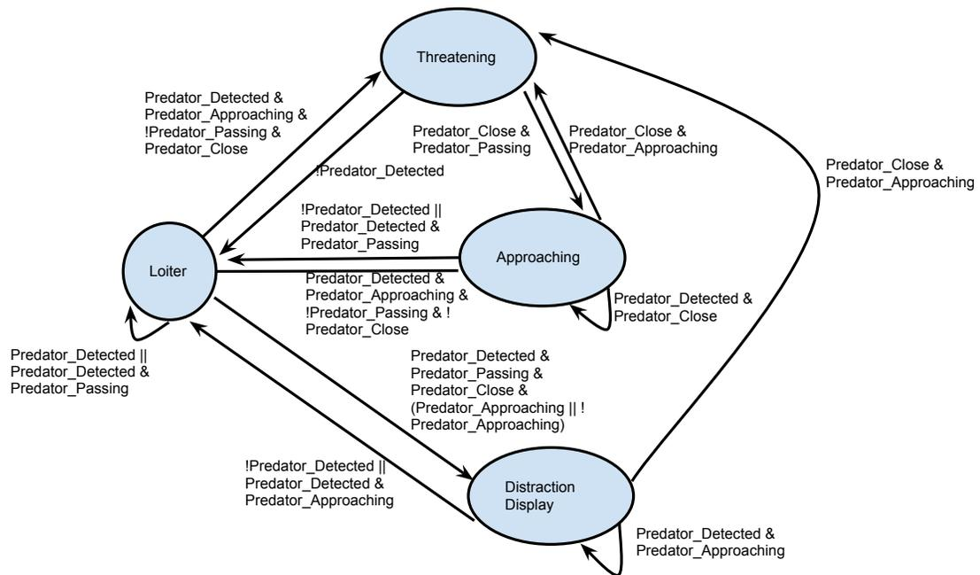
Figure 3.2: A finite state machine depicting the triggering of Site Defense behaviors discovered through a review of literature.
