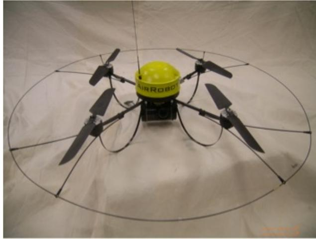
Figure 5.1: AirRobot AR100B platform from AirRobot.
