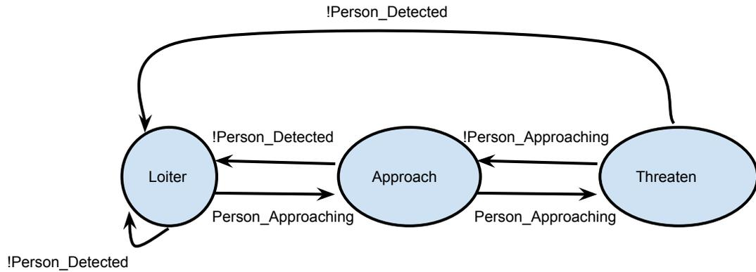
Figure 4.3: Site Defense escalation strategy for robots based on identified behaviors.
