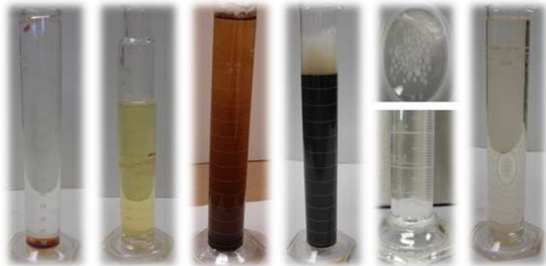
Fig. 33 —Dispersants (from left to right) N60 with oil, N60 with water, N47 with oil, N47 with water, N50 with oil, S2 with oil. Dispersant concentration was 1.6 wt%. Dispersants information in Appendix A.
