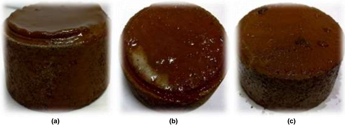
Fig. 48—Two-step procedure to dissolve Mn_3O_4 -based filter cake on Indiana core samples at 250°F: filter cake (a) before removal, (b) after enzyme reaction, and (c) after glycolic acid reaction. The enzyme and glycolic acid concentrations were 10 wt%
