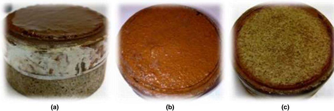
Fig. 47—Two-step procedure to dissolve Mn_3O_4 -based filter cake on Indiana core samples at 250°F: filter cake (a) before removal, (b) after enzyme reaction, and (c) after glycolic acid reaction. The glycolic acid and enzyme concentrations were 5 and 10 wt%, respectively.
