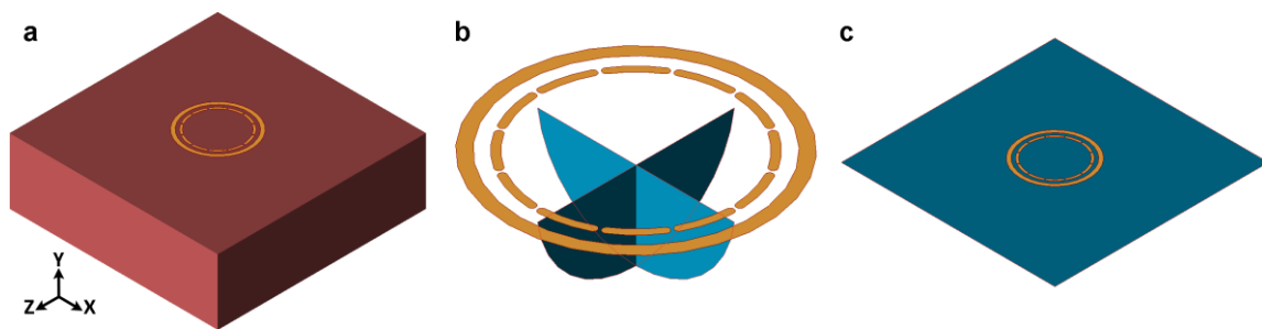
Figure II-1. Renderings of surface coil adjacent to the phantom load and EM field sensors. (a) 16-cm coil with coplanar shield centered over dielectric slab. (b) Sensors 1a and 1b were located on the xy and yz planes, respectively, both orthogonal to the coil and consisting of hemispheres (of the coil radius) excluding the region within 1 cm of the coil. (c) Sensor 2 was a square sensor located 1 mm inside the near face of the slab on the xz plane.
