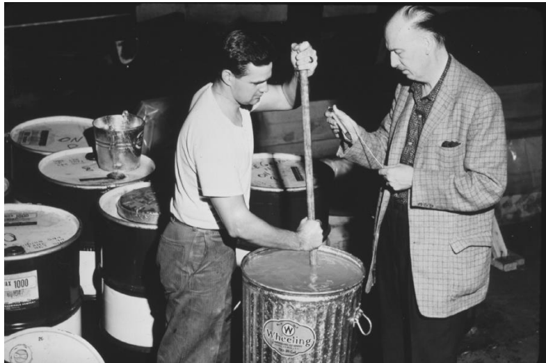
Figure 8. Dr. Robert Inverarity checking a vat of Polyethylene Glycol (PEG) during conservation of the Lake George bateaux. (Photo: Adirondack Museum. 1961.)
