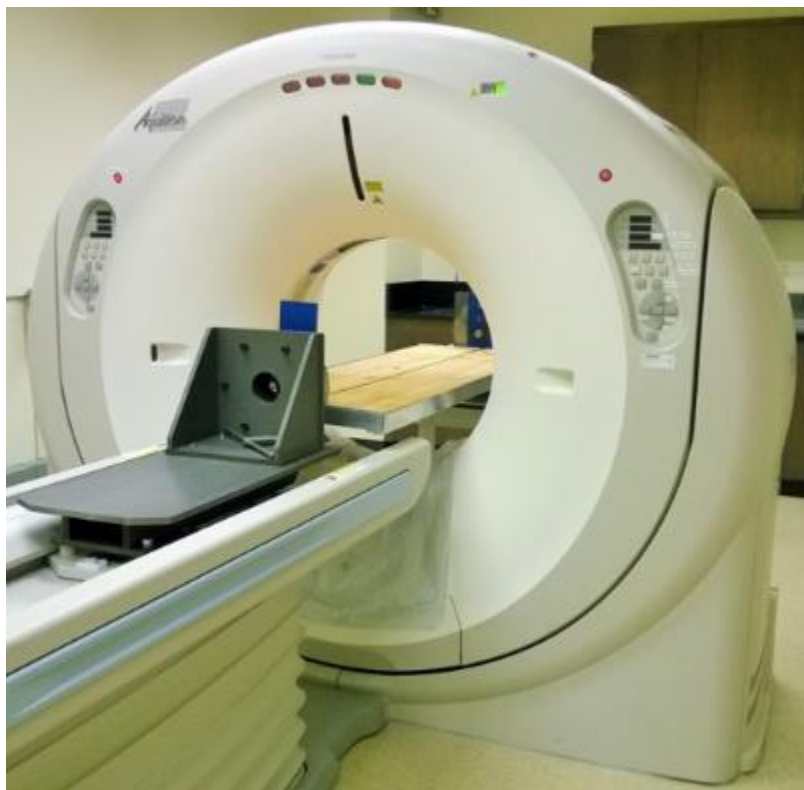
Fig. 3–CT-scanner used to characterize the dissolution structures created by MSA in dolomite cores.
