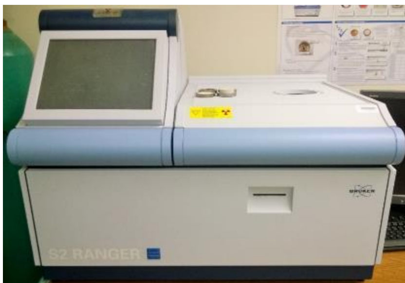
Fig. 5–S2 Ranger X-Ray Fluorescence (XRF).
