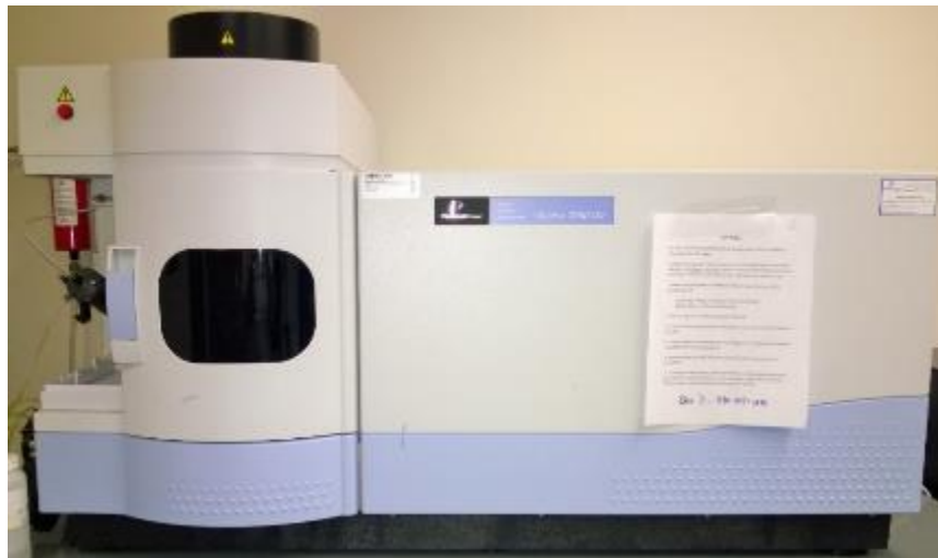
Fig. 4–Inductively Coupled Plasma Optical Emission Spectrometry (ICP-OES).
