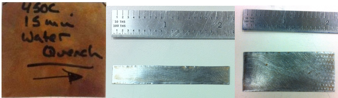
(a) Original raw NiTi (at. 50.0% Ni) Sample. (b) Thin Strip specimen. (c) Plate specimen.
