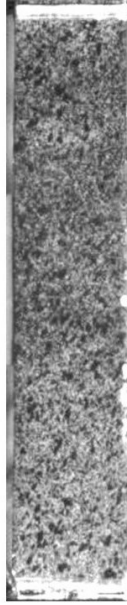
Figure 1.4: An example of a good DIC speckle pattern is shown. The NiTi specimen was painted with a white background and black speckles. A good distribution of similar-sized black speckles was used with a white background.
