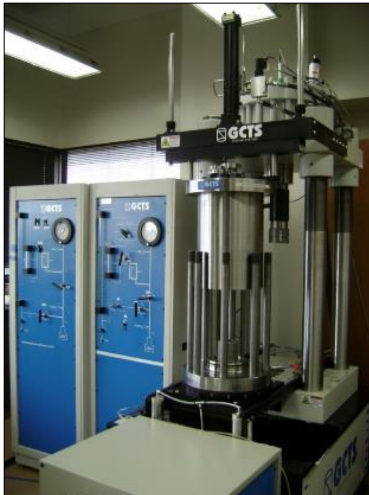
Figure 14: Tri-axial system used to measure bulk and shear moduli in the laboratory.
