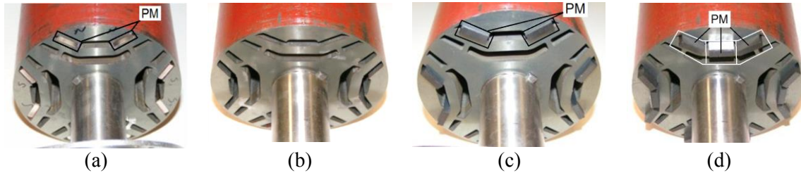
Fig 3-30: Studied rotors: (a) Original rotor with NdFeB magnets, (b) Magnet-less rotor core, (c) PMa-SynRM-C8-R1, (d) PMa-SynRM-C8-R2.
