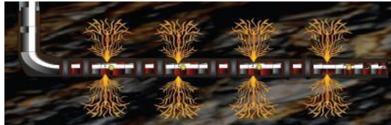
Figure 7: Multi-stage hydraulic fracturing (FracStim)
