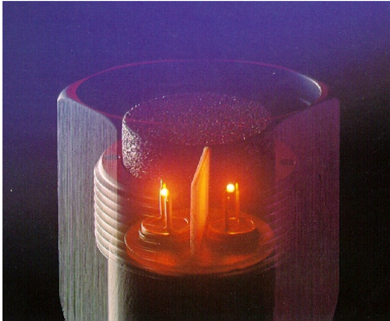
Figure 1.1: Catalytic bead sensor from a gas detector manufactured by Delphian Detection Technologies.
