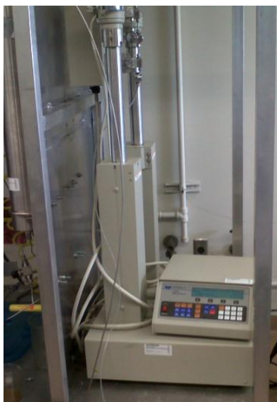
Fig 2.10– Syringe pump. Continuous Flow 260D Teledyne ISCO Dual Syringe Pump and controller
