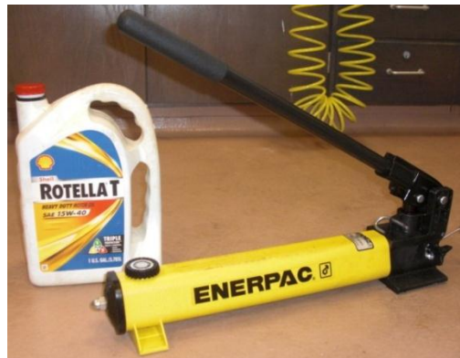
Fig 2.9 – Overburden pump. ENERPAC hydraulic hand pump is used to apply confining pressure on the core.
