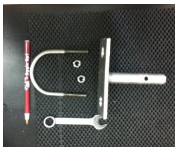
Fig 4.8—Core holder mounting components
