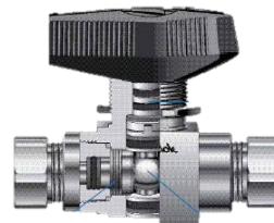
Fig 2.21 – Swagelok 2-way ball valve interior structure
