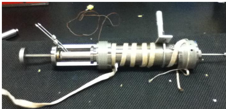
Fig 4.7— Core holder with heating tape
