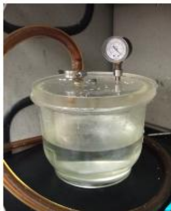
Fig. 4.2-- Saturation cell in lab 821
