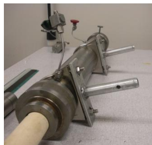
Fig 4.9—Mounting attached to core holder
