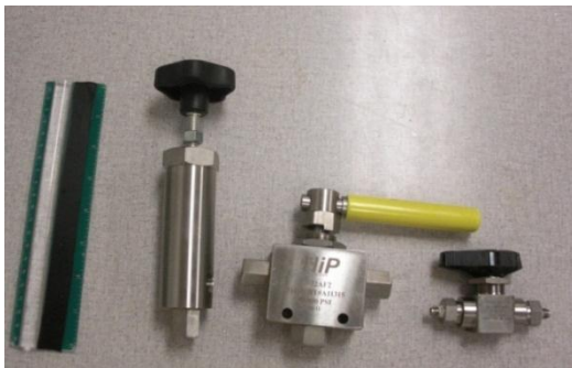
Fig 2.20 – Apparatus valves. From left to right: relief valve, 3-way ball valve, 2-way ball valve
