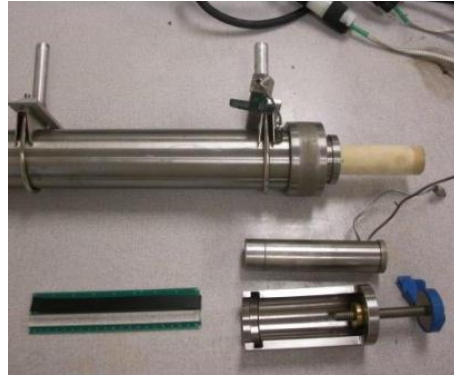
Fig 4.6-- Floating platen, tightening assembly and end cap
