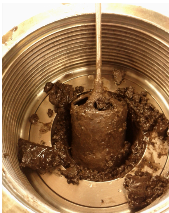
Fig. 4.8 - Failed fluid sample
