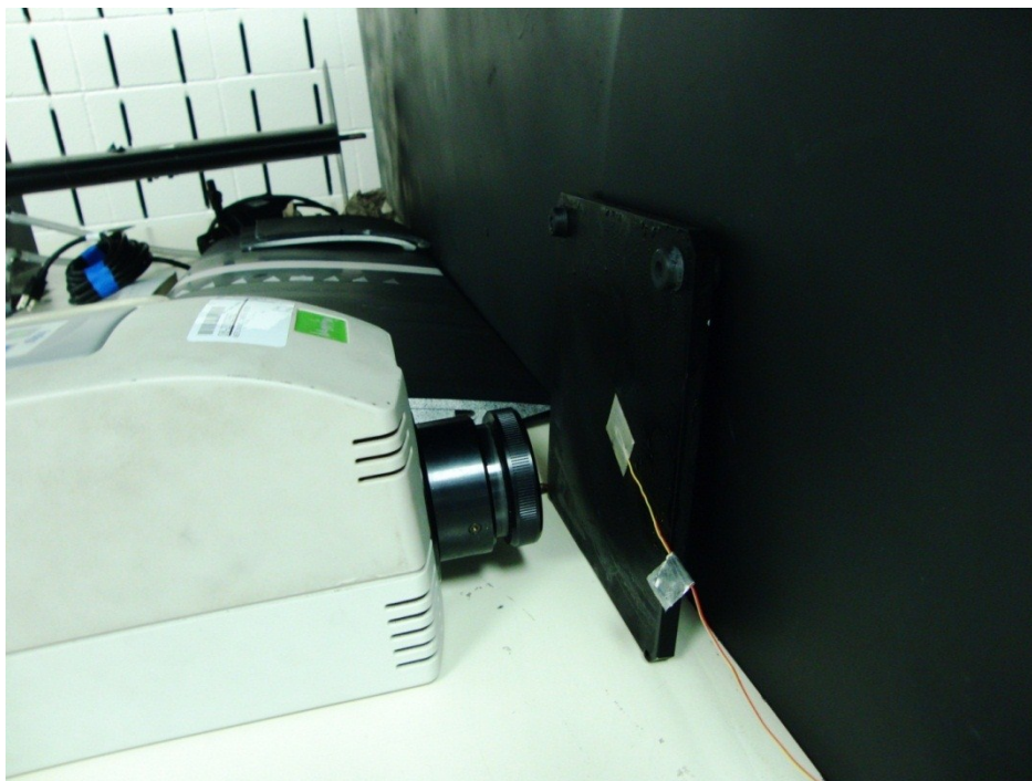
Figure 21 Camera calibration setup, shown with camera away from plate
