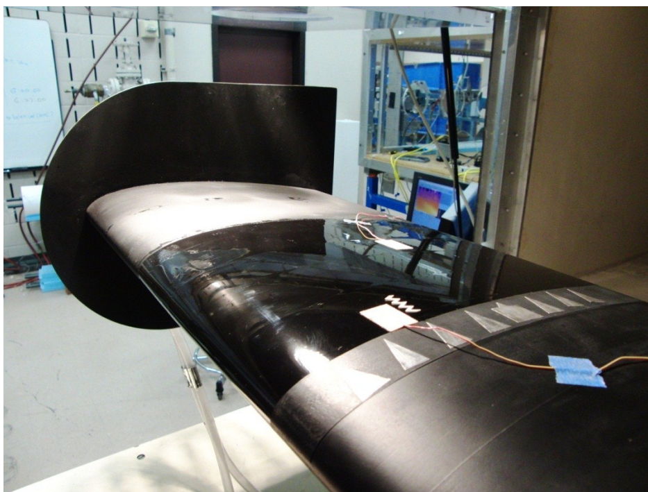
Figure 34 Painted RP plastic test model with Monokote over the layer of Bondo
