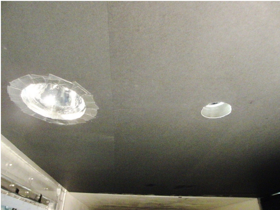
Figure 17 Test section ceiling covered with black paper and showing the lamp mounted in the ceiling hole (left) and the hole cut for the camera (right).
