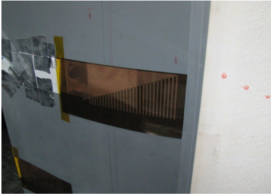
Figure 1 Hotfilm array installed on test wing surface
