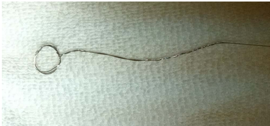
Figure 4: Oral Electrode. Oral electrode constructed out of stainless steel suture; circular portion to be positioned around the tongue of the test subject, straight end attached to output pin of the precision current source via alligator clip.
