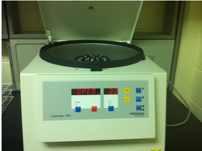
Figure 9: Centrifuge. Clotted samples were centrifuged, then serum to be tested for octreotide concentration was extracted and stored in the -20 degrees Fahrenheit freezer
