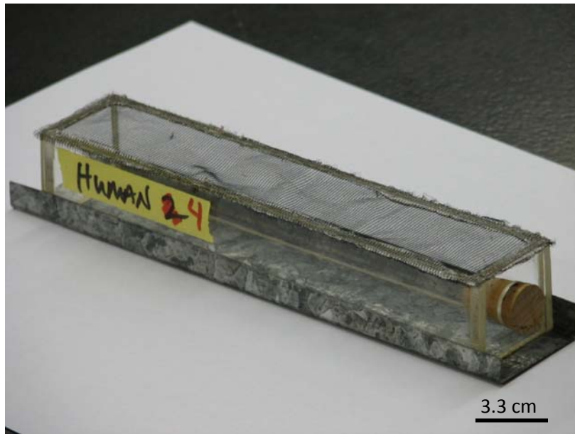
Figure 4.2. Image of the mosquito blood-feeding cage. The mosquitoes are introduced through the stoppered hole and mosquitoes can feed through the screen. When feeding is complete the metal bottom slides off to release the mosquitoes.
