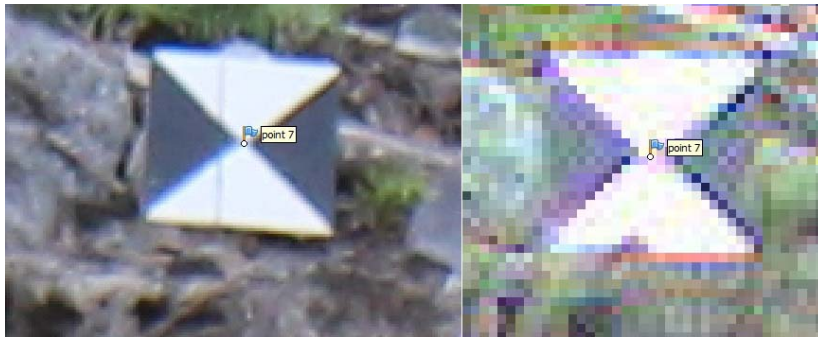
Fig. 61. 18MP Sensor from Canon Rebel T2i (Left) vs 3.1MP Sensor in Reconyx time-lapse capsules (Right). Even though image quality is poorer and resolution is lower, the images from the Reconyx capsules created a more accurate DTM.
