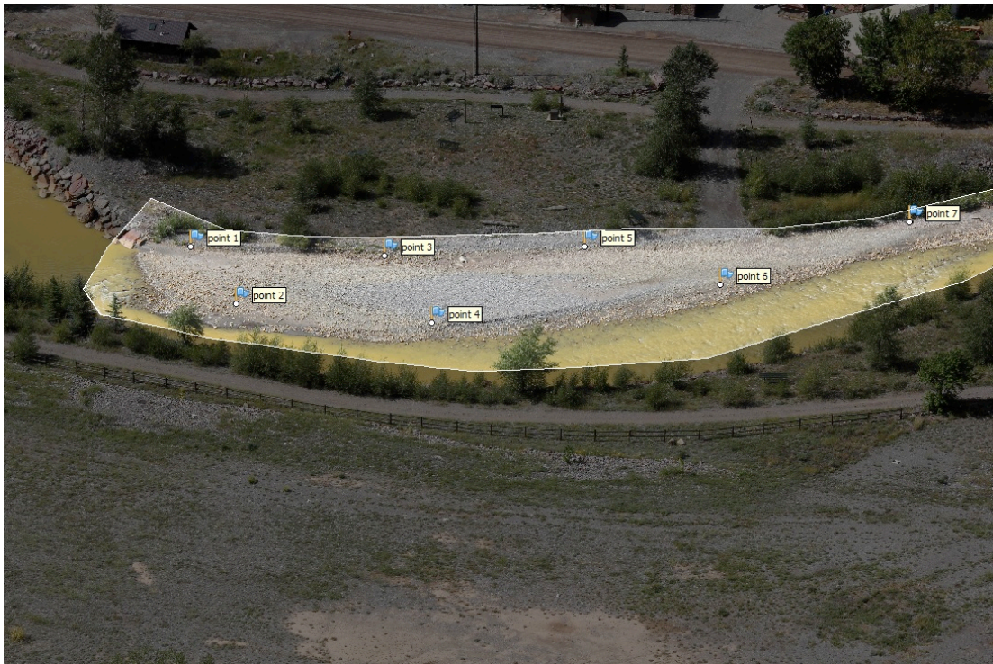
Fig. 47. Screen shot of image used in DTM processing with an image mask only covering the gravel bar. Nine ground control points (GCPs) in total were located on the gravel bar in September.
