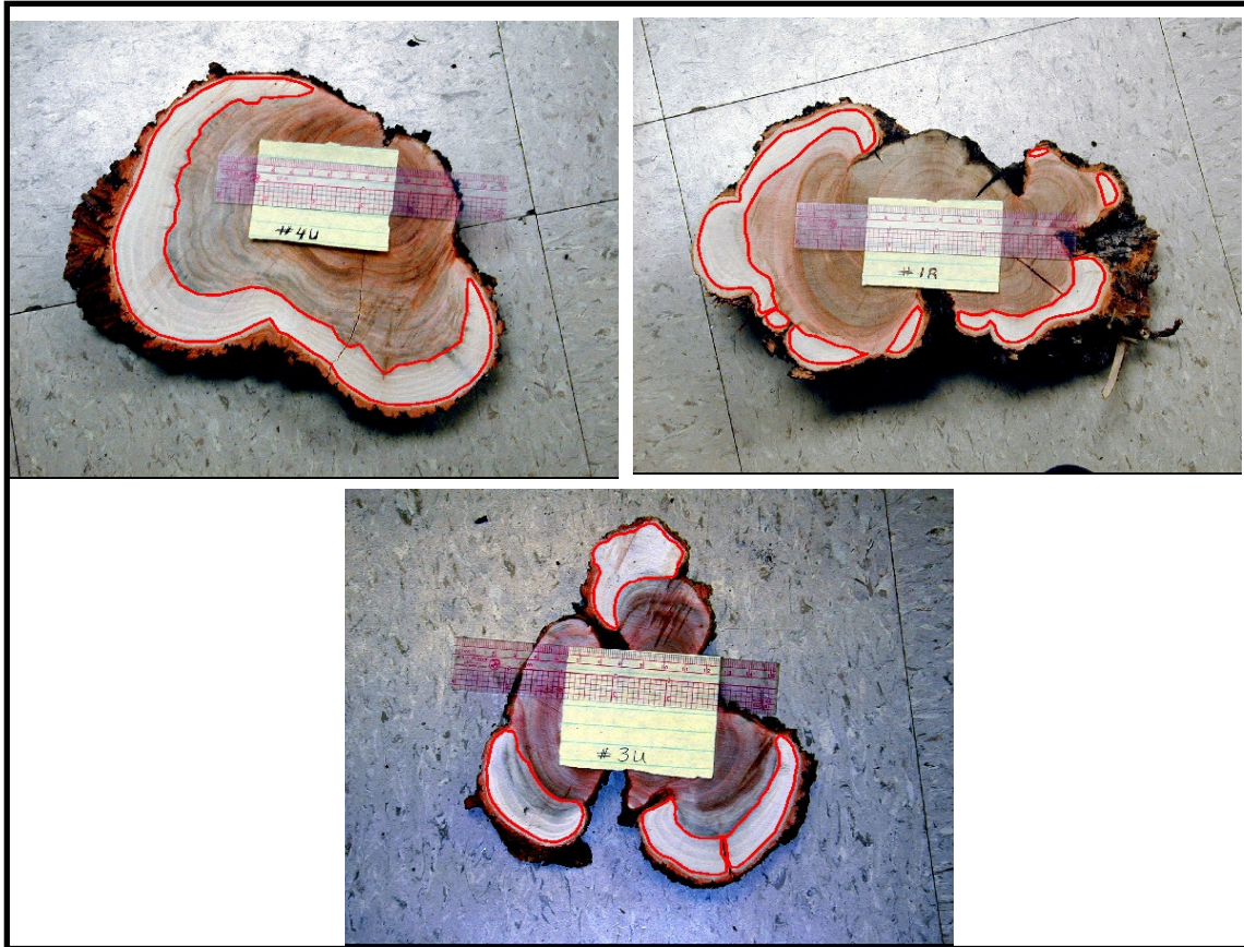
Figure 3.1 Photos of saltcedar stump cross sections, and delineation of sapwood area, harvested from the PREP study area along the Pecos River, Texas.
