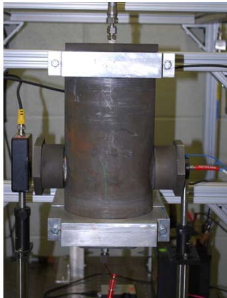
Figure 9. High-pressure strand burner at Texas A&M University.
