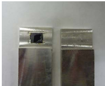
FIG. 26. Test sample after pressing with minimal force and temperature.
