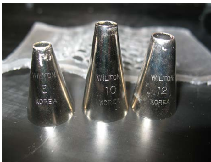
Fig. 3.2. Cake tips used for punching out PDMS discs.
