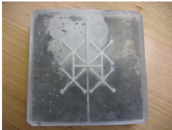
Fig. 7.13. Damaged fluidic network.
