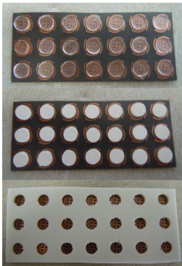
Fig. 4.7. 3 by 7 FSS with PDMS discs(top), BSTO in PDMS discs at \phi=40% (middle), Silicone Oil foam tray(bottom).
