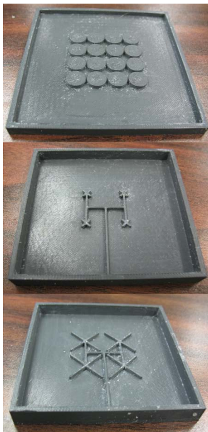
Fig. 7.6. Master molds for fluidic network PDMS layers.
