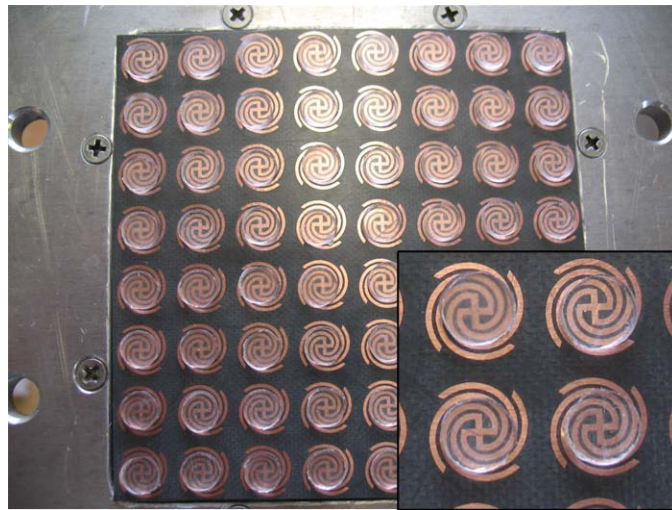
Fig. 6.1. Close up of PDMS discs on spirals.
