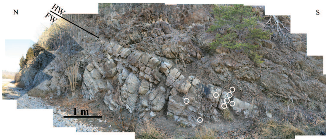
Figure 2. Exposure of the CC thrust fault. Copper Creek thrust fault 32 km north of Knoxville, TN. The footwall (FW) is composed of shale and micrite beds, while the hanging wall (HW) is composed of shale, carbonate, and sandstone beds. The hanging wall is displaced to the north. Samples taken near the FW-HW contact (circles).
