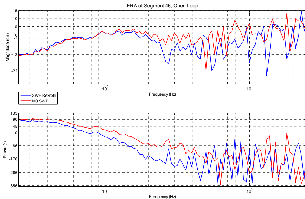
Fig. 17. FRA for Paddle 45, h=0.50 m, Open Loop, Alpha = 0, with and without SWF from Rexroth
