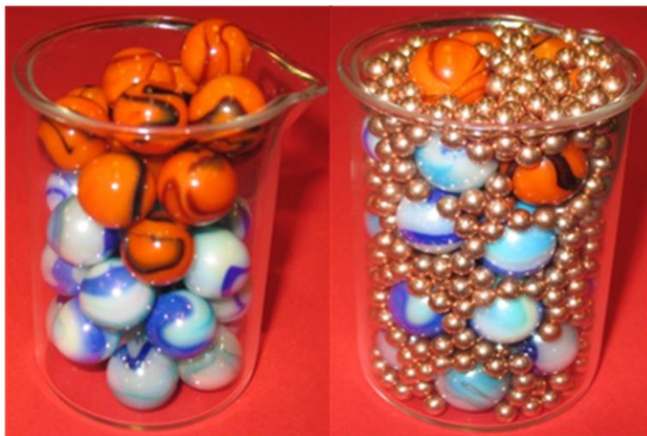
Fig.3. Photos demonstrating a monodispersed system of spherical particles using marbles (left) and polydispersed particles using a mixture of marbles and BB's (right).
