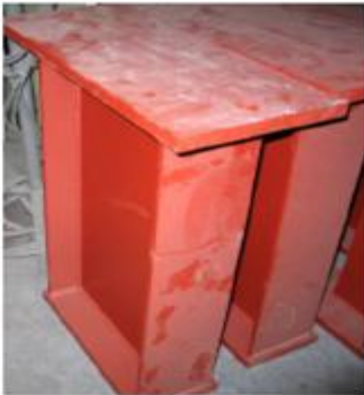
Figure 2-2: 33 1/2" tall pedestal with dimensions of the top plate [1]
