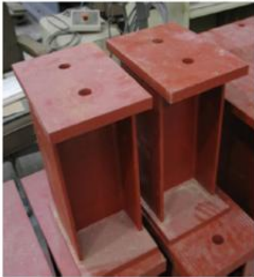
Figure 2-1: 19" tall pedestals with dimensions of the top plate [1]
